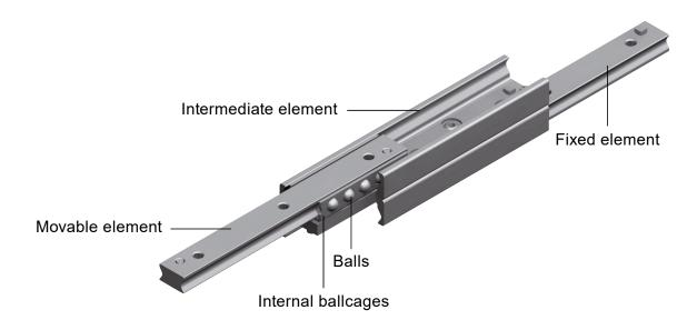
The Telescopic Rail Heavy range consists of versions with full and partial extension and various cross-sections and intermediate elements in S-shape, double-T or square. High loads in combination with cost-efficiency and free movement have long been the outstanding properties of the telescopic rail product line.
