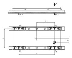
Note: It is defined that the slider no. 4 is always located closest to the point where the force is applied.
