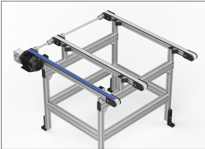
Single conveyor general load limits depend on the maximal torque the drive shaft can transfer to the drive wheel. For short conveyors, the load per meter may be the effective limit. See [Table 1](#) and [Table 2](#).
