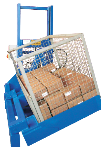
Lift system, hydraulic.
